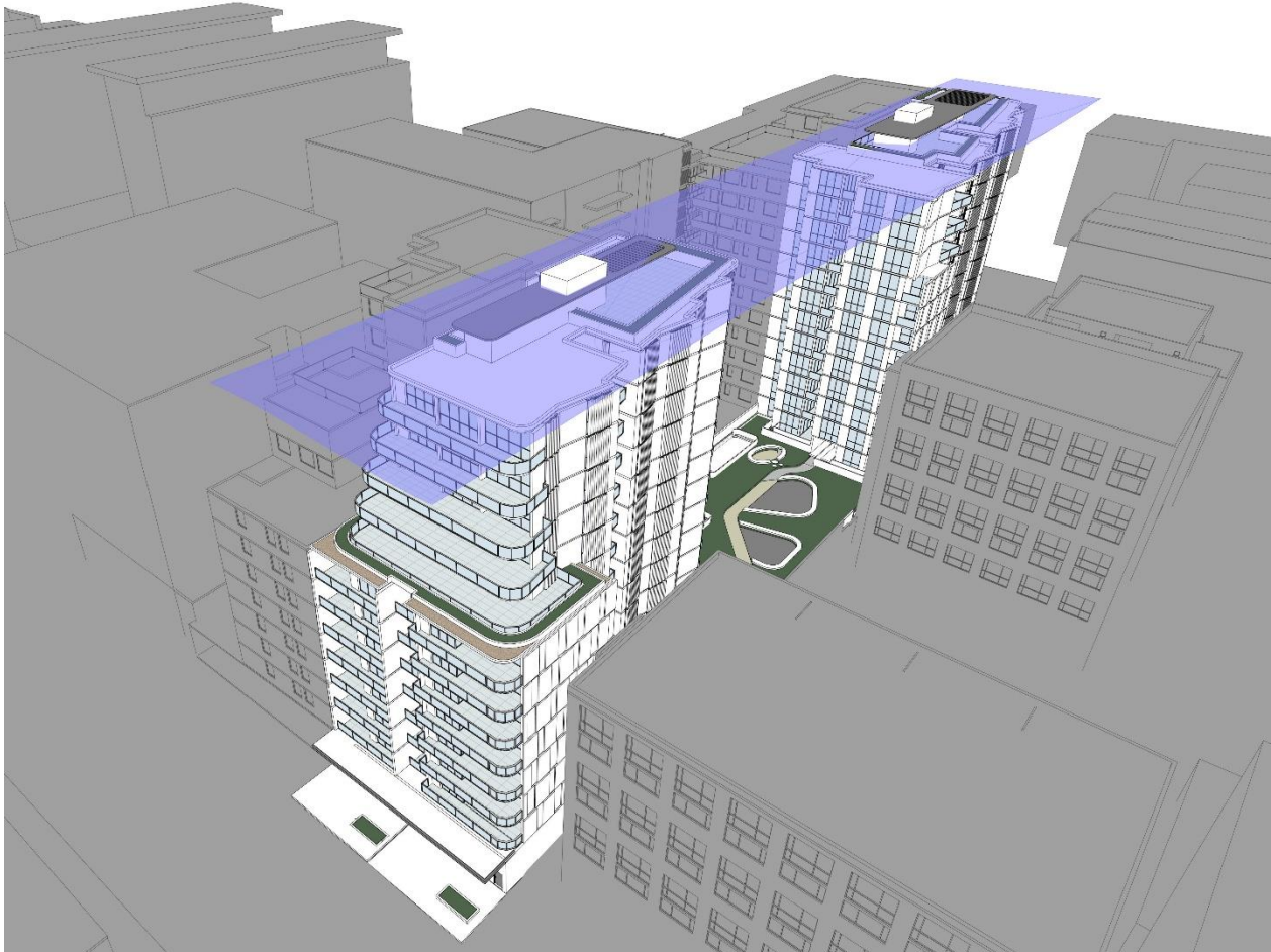
Figure 2 Diagram illustrating building height control and area of non-compliance at Building A and B
